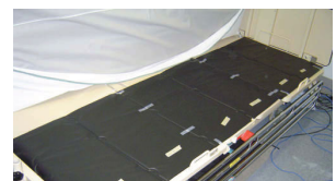
Figure 1: Hospital bed with pressure sensor array (mattress is placed on top)
